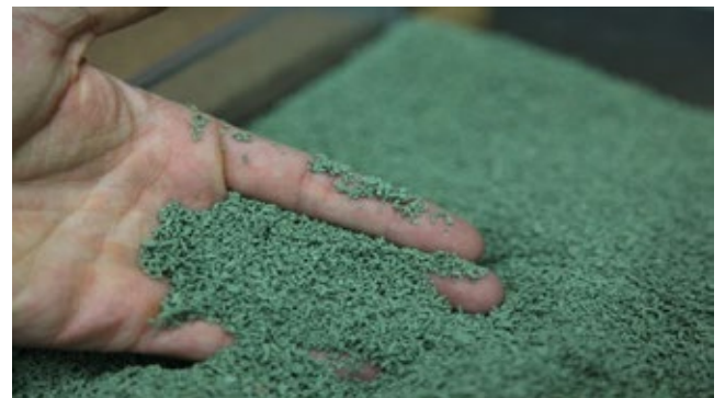
Photo 12: EPDM 'Bionic' infill (Source MELOS)
